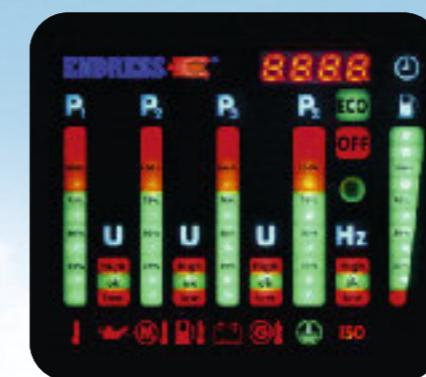
A light sensor controls the LEDs on the basis of light incidence so that good visibility is guaranteed even in direct sunlight.
